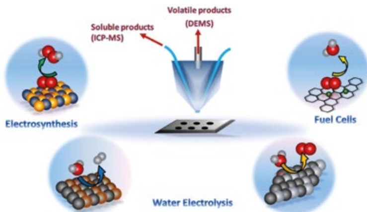
Fig. 11: Schematic overview of the applications of a flow cell coupled to analytics for simultaneous detection of soluble and volatile reaction products and intermediates in energy conversion related applications such as fuel cells and electrolysis. On-line ICP-MS (inductively coupled plasma mass spectrometry) allows precise quantification of dissolution in electrochemistry, while DEMS (differential electrochemical mass spectrometry) enables qualitative analysis of gaseous species formed during the reaction.
